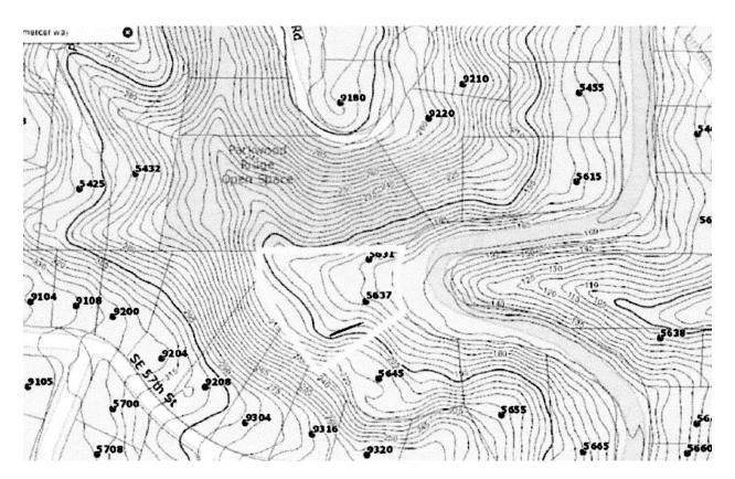
The black line superimposed on the map is the approximate location of the southeast wall of the proposed residence. The slope to the southeast of the residence is relatively mild compared to the very steep slopes south and southwest of the residence.
